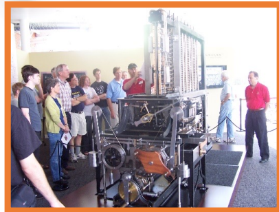
1832, 2002, 2008 The Babbage Difference Engine, 17 years, 25,000 parts, 5ton, cost: £17,470
